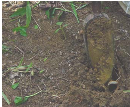
Uplift the auger with all its content of soil.
