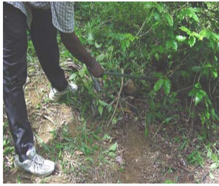
Collect sample between rows and not at the root of the plant.
