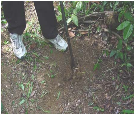
Turn the auger clockwise and lower it to the neck or about 8 inches.
