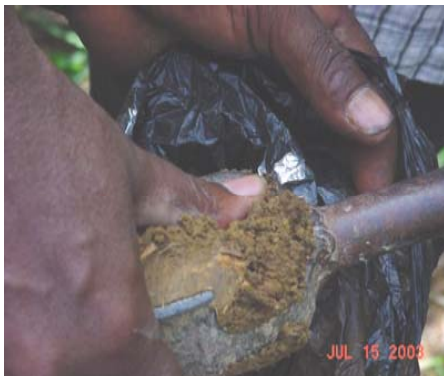
Clear the soil from the auger in a container; bag, box, etc.
